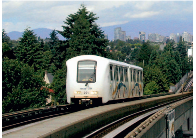
Fig. 1. Transport system using linear induction motor (LIM) technology. Canada
