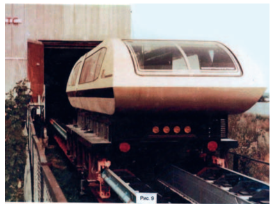
Pic. 5. Testing of 18 ton TP-05 car using traction electric linear motor and magnetic suspension
