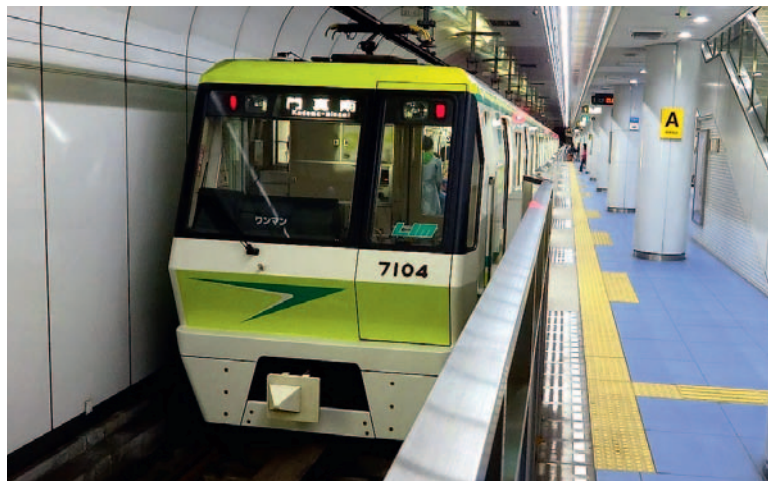
Fig. 2. Subway line using LIM technology. Japan
