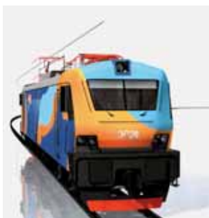
EP20 passenger double-current electric locomotive with asynchronous traction drive (Novocherkassk Electric Locomotive Plant — Alstom)
