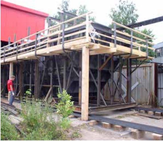
Fig. 8. Moulding tools for the hopper underframe
