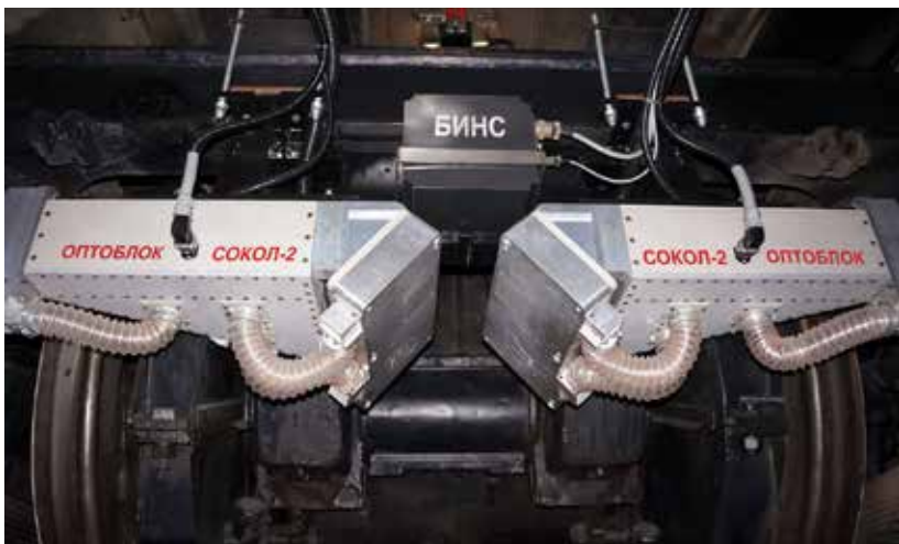
Fig. 2. SOKOL-2 track geometry assessment system
