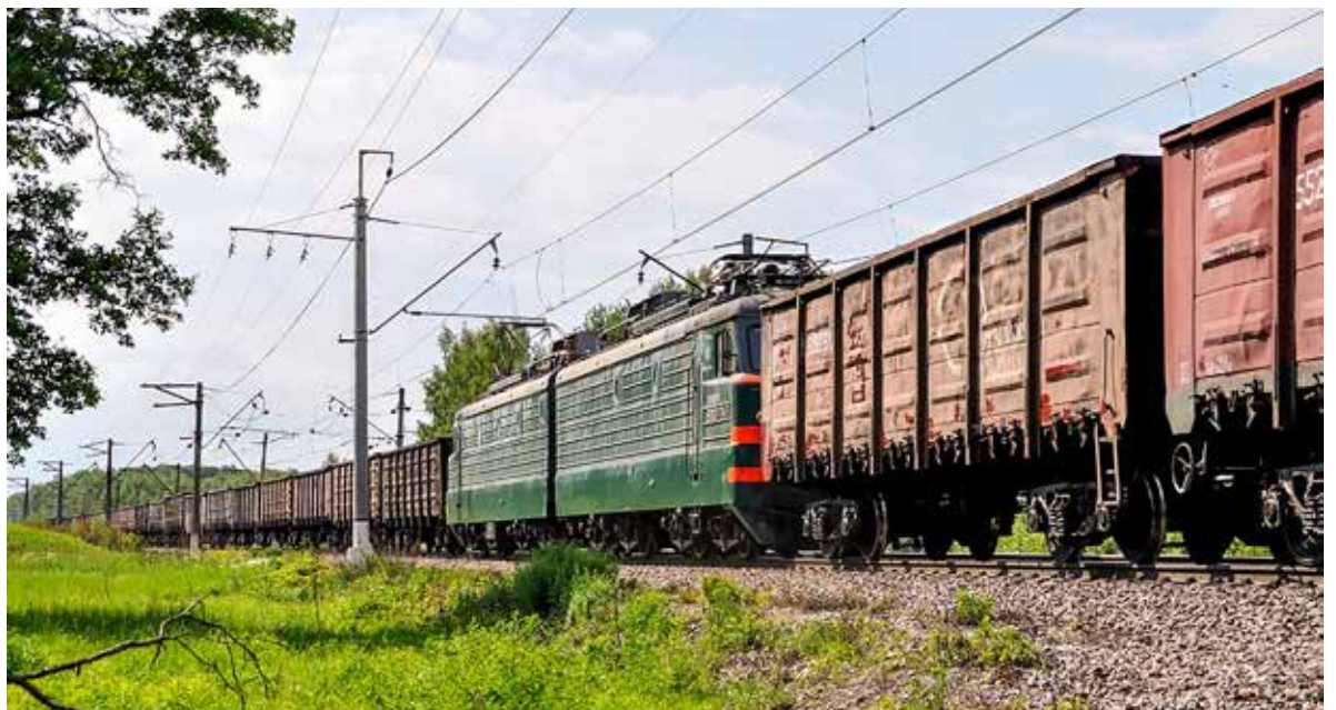
Fig. 6. Joint trainsets running in automatic control mode (ISAVP-RT) with distributed power
