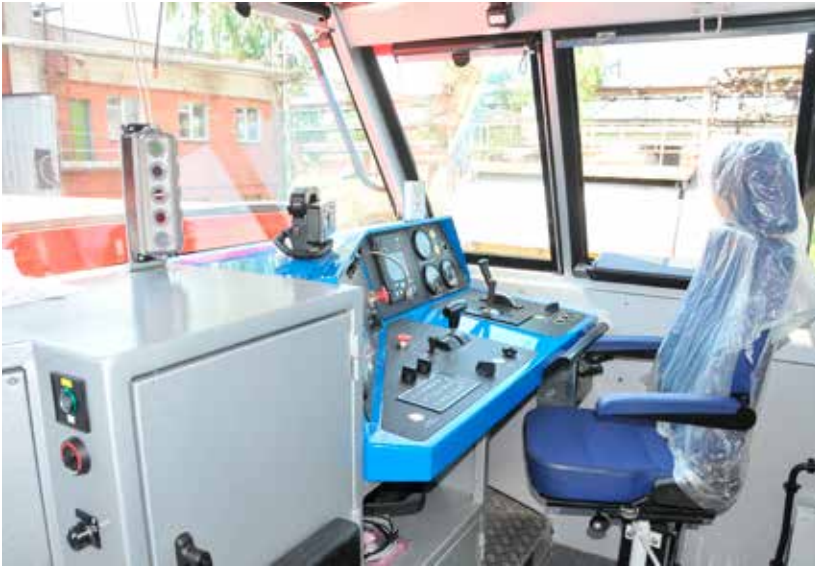
Fig. 4. TEM35 is operated by a single driver eliminating the need for a driver's assistant
