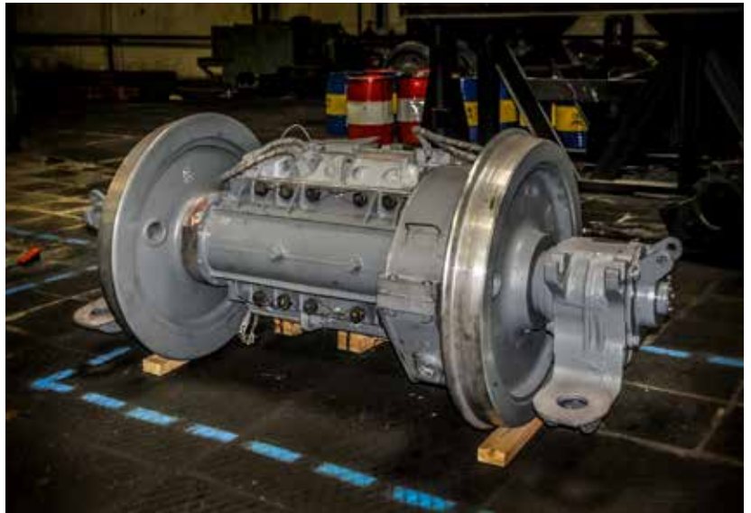
Fig. 3. Wheels-and axle subassembly consist of a DC traction motor and a standard design wheelset with an antifriction axle hung bearings designed by BMZ CJSC engineers.
