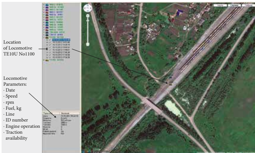
Fig. 3. Tracking and condition monitoring of the locomotives equipped with ADS and Event Recorder is based on data sent to the server via wireless links
