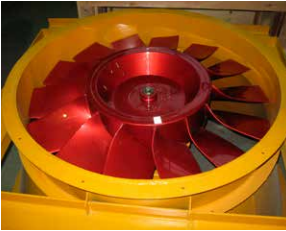
Fig. 3. Cooling Ventilator with Bar Blades
