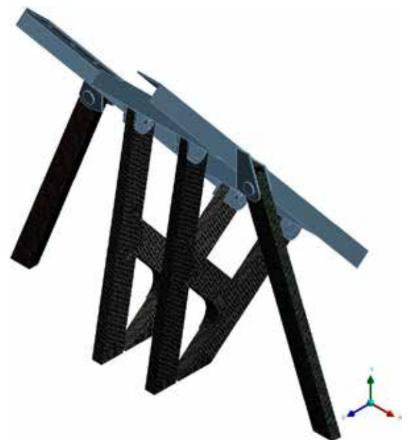
Fig. 5b. Finite element models of hopper end walls diagonals
